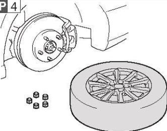
Remove all the wheel nuts and the tyre. When resting the tyre on the ground, place the tyre so that the wheel design faces up to avoid scratching the wheel surface.
