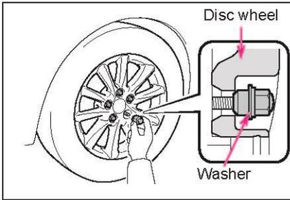
When replacing an aluminium wheel with an aluminium wheel, turn the wheel nuts until the washers come into contact with the disc wheel.
