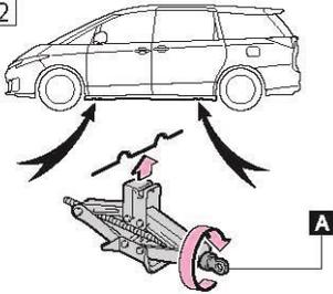
Turn the tyre jack portion "A" by hand until the notch of the jack is in contact with the jack point.
