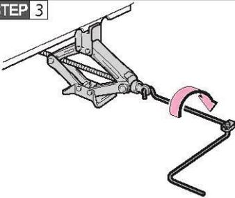
Raise the vehicle until the tyre is slightly raised off the ground.
