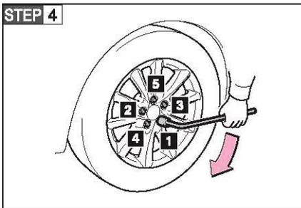
Firmly tighten each wheel nut two or three times turn clockwise in the order shown in the illustration.
