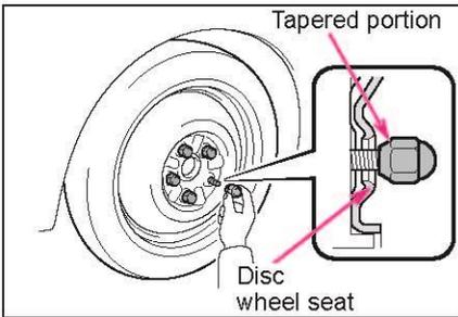
When replacing a steel wheel with a steel wheel (including a compact spare tyre), tighten the wheel nuts until the tapered portion comes into loose contact with the disc wheel seat.
