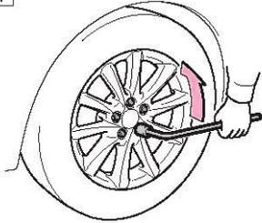
Slightly loosen the wheel nuts, turn anti-clockwise (one turn).
