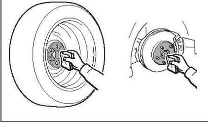
Remove any dirt or foreign matter from the wheel contact surface.
