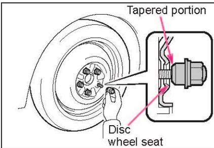
When replacing an aluminium wheel with a compact spare tyre, tighten the wheel nuts until the tapered portion comes into loose contact with the disc wheel seat.
