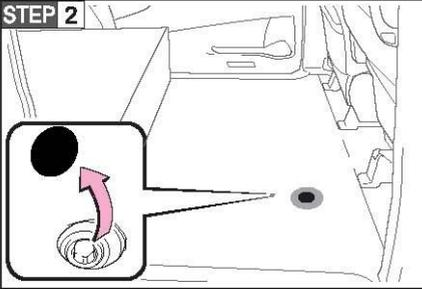
Pull out the black cap to find the spare tyre clamp bolt.
