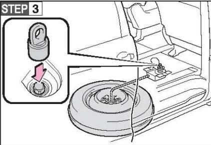
Attach the adapter socket to the spare tyre clamp bolt.
