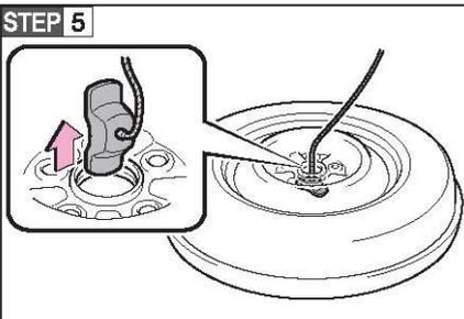
Slide the compact spare tyre out from underneath the vehicle and remove the holding bracket.
